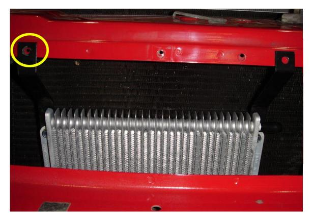
With the top of PWR cooler brackets now secure, proceed to drill a pair of 6mm holes to align with the lower bracket holes as circled.
