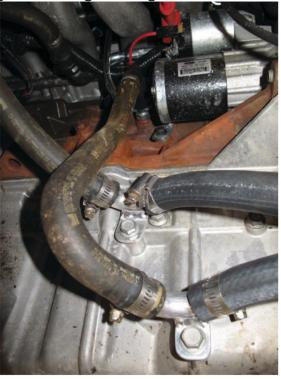
Pre-filling the transmission oil into the lines of the heat exchanger is recommended to minimise any possible air locks or bubbles inside the heat exchanger. A hand operated oil pump/syringe may assist in this procedure.
