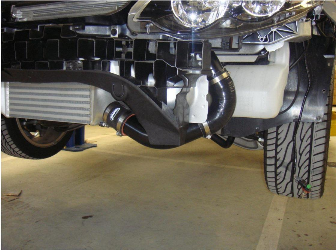
Working our way to the left side of vehicle, proceed to feed **item no.11** though under head light and leave hang there.
