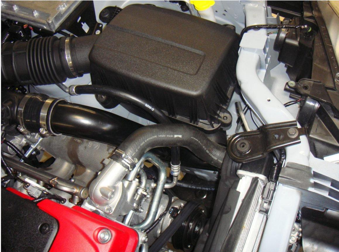
Fit silicon hose **No.12** to end of pipe entering engine bay (**pipe item No.11**)
