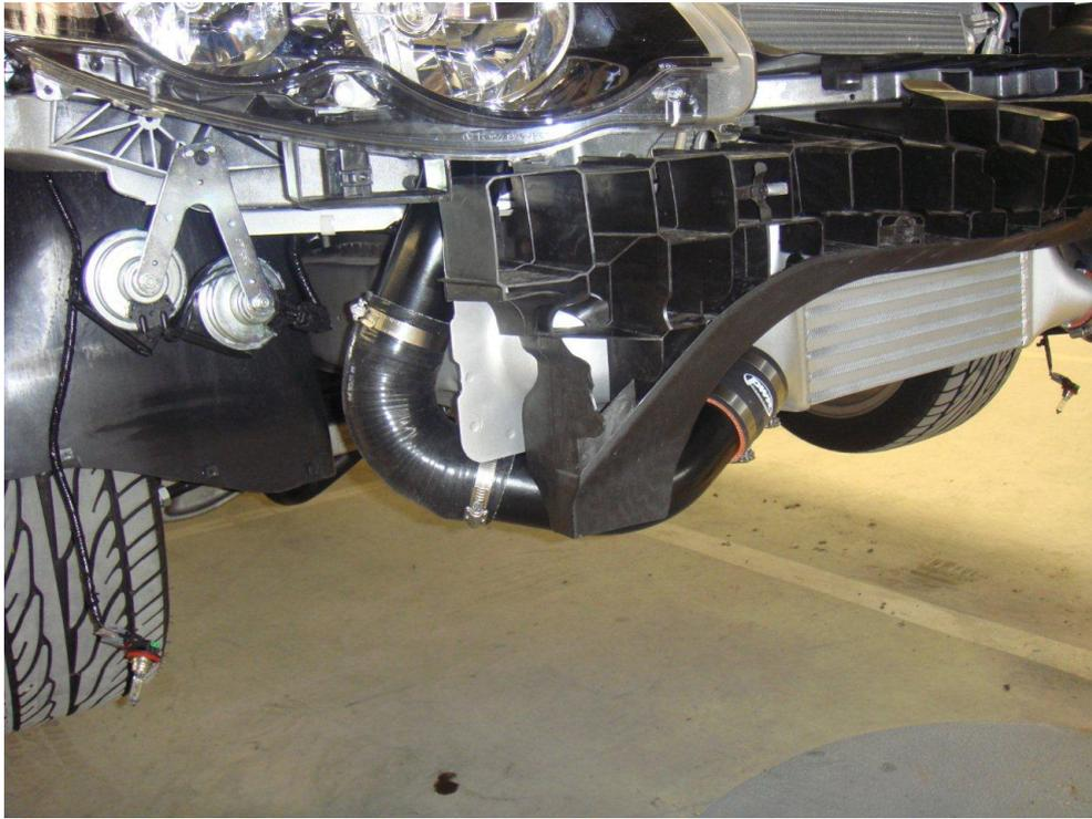
Connect Pipe Item **No.6** and Item **No.7** placing a 2.5 hose clamp on each as pictured . Keep in mind to align the hose clamps for ease of access to tighten. Tighten each clamp.
