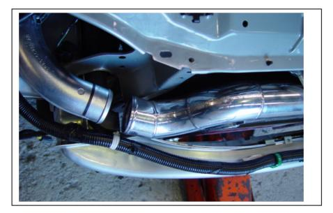
8. MODIFYING OF THE FORD BRACKET ON THE LEFT HAND SIDE IS REQUIRED TO ALLOW CLEARANCE OF THE NEW THICKER INTERCOOLER. WITH THE BRACKET SECURED IN A VICE AND CUT ALONG THE LINE AS SHOWN DIAGRAM.
