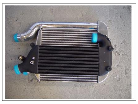
5. COMPARING OF THE PWR INTERCOOLER TO THE FACTORY FORD UNIT WE CAN SEE THE ARE IS OVER DOUBLE AREA AND THE TUBE COUNT IS AT 21 PWR AGAINST 8 ON THE ORIGINAL UNIT.
