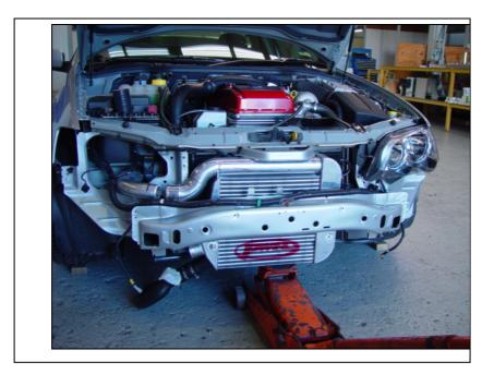
7. SUPPORTING THE UNIT WITH A JACK IS EASIEST. THE ALIGNMENT OF THE TOP HOSE SHOULD LOOK LIKE THIS
