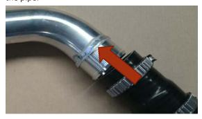
Be sure to push the silicone all the way on to the pipe up to the shoulders. Once in place tighten firmly and check it is secure and will not rub on anything.
