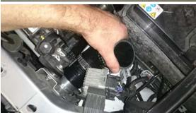
Push the 67-degree lower silicone bend on to the intercooler first then push on the 2.25 – 2.5 inch silicone at the throttle body end of the pipe.
