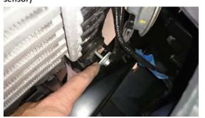
24. Remove intercooler and place aside for disassembly.
