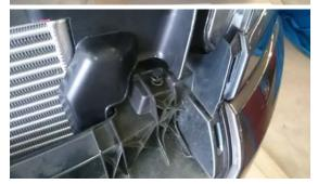
35. Reinstall the 2 pushpins in the top of the bumper.
