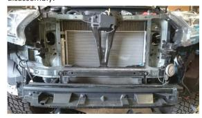
25. Undo the screw using a T-25 Torx bit that is holding the sensor in the intercooler. Remove the sensor and set aside for reinstallation discard the screw. (Be sure to clean any dirt away before removing the sensor)
