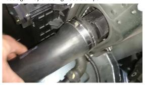
20. Undo and remove the radiator air ducting (2 places each) using an 8mm socket and retain for reinstallation.
