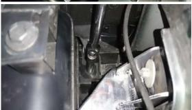
7. Using a T-25 torx bit undo the 2 screws at the bottom of the grille retaining it to the bumper.
