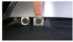
38. Reinstall flares (if fitted) and secure the bumper the original clips and screws.
