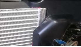
32. Once the plastic is trimmed and the fit is snug use the factory bolts to reinstall the ducting to the vehicle.
