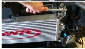
30. The supplied spacers (99A18985) may need to be placed behind the intercooler to ensure adequate clearance of approximately 3mm from the Intercooler core to the radiator core support panel area as highlighted in images below with arrow.
