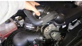
19. Undo and remove the bottom intercooler inlet hose again by undoing hose clamps.
