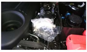
18. Loosen the 2 clamps on the air box intake tube and pull the tube up and out of the way.
