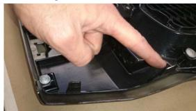
41. The 4 original bolts can be secured from the top using a 10mm socket.
