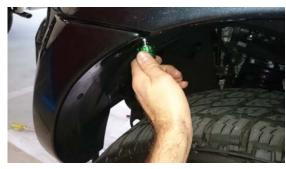
11. Remove the 4 bolts from under the bumper using a 10mm socket. Retain for reinstallation.
