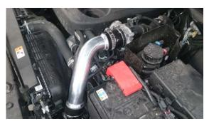
Remove hot OEM hose as per step 18 and 19 in section 1. Ensure that you have removed any tape or rags from inlets and outlets
