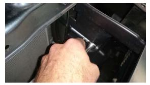
21. Undo clips for air temp sensor on the bottom of the duct as shown
