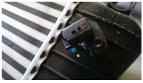
26. Remove the rubber mounting grommets from the OEM intercooler and place aside for reinstallation into the new PWR intercooler.
