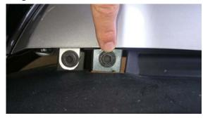
12. Unplug the fog lights (1 plug each side) and unplug driving assist sensors if fitted (1 plug under passenger side).
