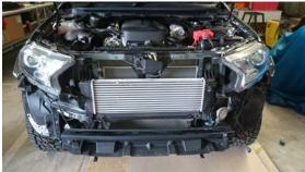
16. Remove the top intercooler hose by undoing the clamps.
