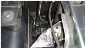
42. The lower 2 screws require the T-25 Torx driver.
