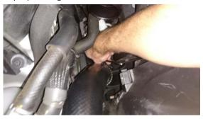
Push the top PWR supplied silicon hump hose onto the Intercooler and then push the lower silicone hump hose onto the lower OE pipe running from under the engine. (This is a firm fit to avoid pipe blow off).
