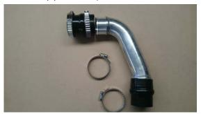
5. Then push down firmly with the aluminum pipe into the silicone. Be sure to push the pipe all the way to the shoulder of the outlets but not past the shoulder
