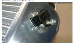
29. Taking care not to damage the core install the new intercooler paying attention to making sure the lower foam strip is in contact with the radiator core support as per next image. Using the original nuts and bolts secure the intercooler into place.
