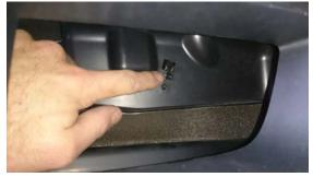
34. Reinstall the front bumper being sure to clip in under the head lights firmly.
