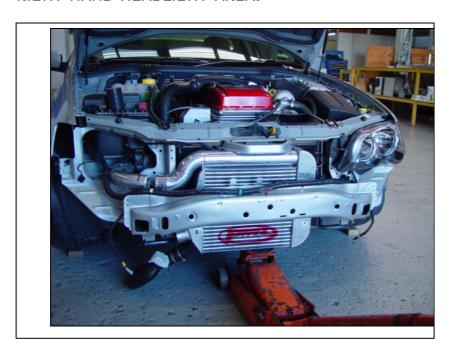
7. SUPPORTING THE UNIT WITH A JACK IS EASIEST. THE ALIGNMENT OF THE TOP HOSE SHOULD LOOK LIKE THIS
