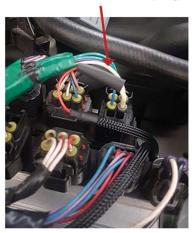
(This will connect ignition to the relays enabling the fans to be only switched ON with ignition.)
