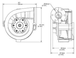
The EWP<sup>®</sup> is a recirculating pump which is ideal for a 'closed system' similar to an automotive cooling system; it is not 'self-priming'. Page 14
